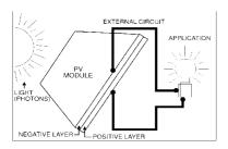
WHAT CAN IT SUPPLY? PV panels are usually used to charge 12v batteries for a wide variety of uses from telecommunications and navigation systems, remote third world villages to caravans, holiday cottages and boats. Single panels are available in sizes from 5 Watts to 170 Watts and can be connected in parallel to give higher currents or in series to produce higher voltages. (Note: when connected in series panels must be of equal current rating).
